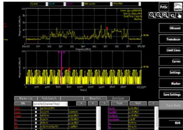
Fig. 2 – Measurement of communication signals (Spectrum, zero span and measurement functions).
