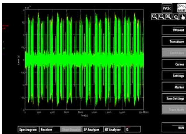
Fig. 6 – Measurement of an amplitude modulated signal as I-Q visualization.
