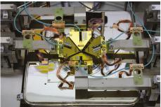
Test of wafer with four Multi |Z| Probes®.
