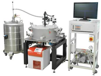
window made of quartz glass contains flanges for vacuum-tight mechanical feedthrough drives. Thus the chuck and up to six vacuum-type positioners can be easily operated from outside via cardan shaft. The high-vacuum pumping system consists of a wide-range Turbo-Molecular Pump (TMP), a diaphragm forepump, and a full-range vacuum gauge. The independently-cooled cryogenic shield ensures ice- and condensation-free probing.
