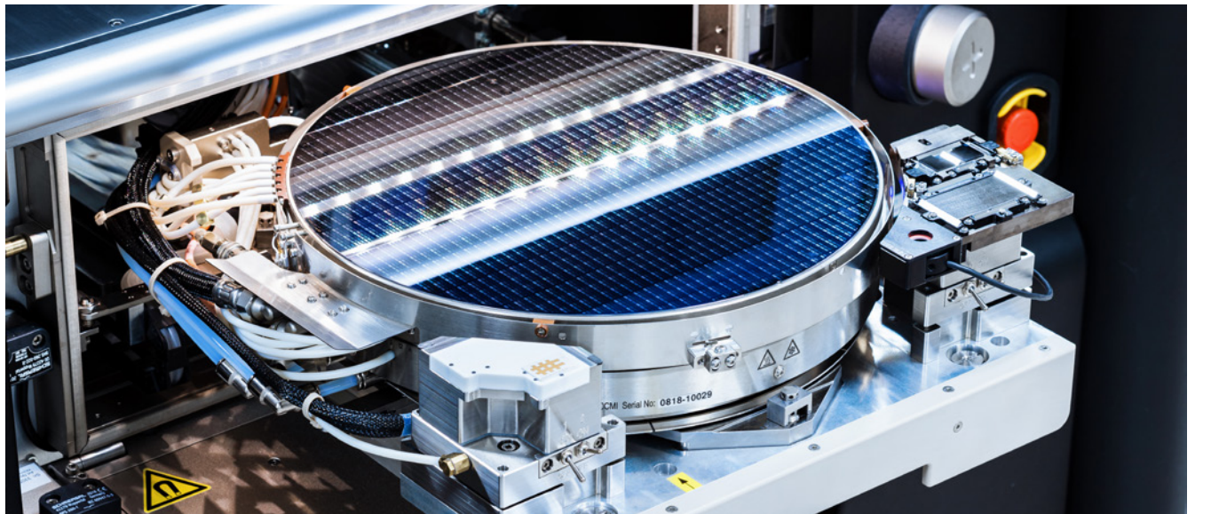
Pull-out chuck with OptoVue Pro in the auxiliary chuck position
