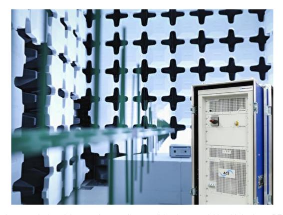
Already at their noteworthy launch in 2013, the versatile, powerful and easy scalable grid simulators **REGATRON TC.ACS** offered almost unlimited possibilities for the simulation of grid conditions and grid disturbances. Easy programming of curve shapes as well as entire waveform sequences and stimulus signals were already standard at that time.
