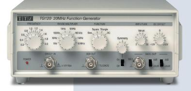
The TG120 uses a different waveform generation technique from that used in other Aim-TTi analog function generators.
