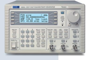
The TG4001 provides high purity sine waves at up to 40MHz and square waves at up to 50MHz. The output amplifier has a bandwidth approaching 100MHz ensuring that waveform quality is excellent right up to the frequency limits. Amplitude flatness is better than  $\pm 0.2$ dB to 1MHz and  $\pm 0.4$ db to 40MHz.
