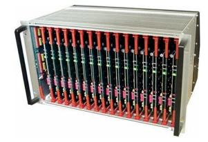
Figure 1: Shows MCOR crate load with 16 Power Modules and interface card on far left.
