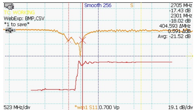
Figure 6: TDR and S11 return loss plots of a 2.4 GHz WiFi patch
