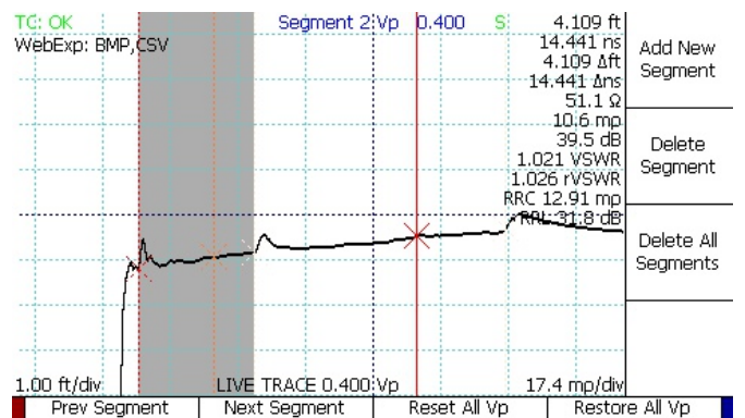
Figure 4: Multisegment cable with first segment VoP of 0.400.
