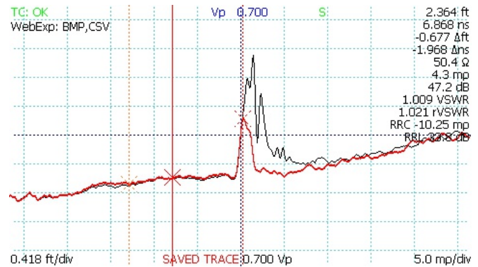
Figure 1: Comparison of normal BNC (black) vs SMA (red) connectors.
